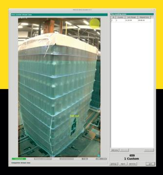
A bottle production company needed a solution which prevents the packaged bottles to be sent to clients unproper foiled. The main problems are due to wearing of the foiling machines or due to uneven thickness of the used foil which leads to random cuts. These cuts leaves some bottles unprotected and they can slip away or can be damaged during the transport stages.
