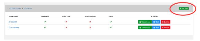
The alarm can be set to be active or not and you can choose one or all of the three types: an **email alert,** a **SMS message** on a phone number if a GSM module is attached to the server, or a **HTTP request**.
